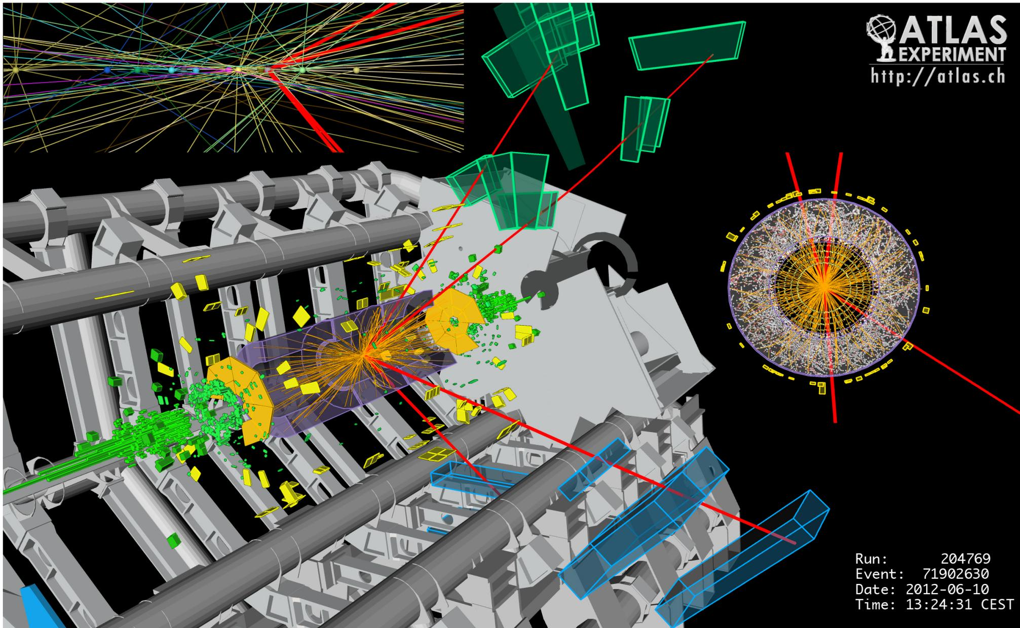
**ATLAS: Candidate event for the decay of a SM Higgs boson into 4 muons (in red). The origin of the 4 muons is a common primary vertex. ATLAS Experiment © 2012 CERN.**
